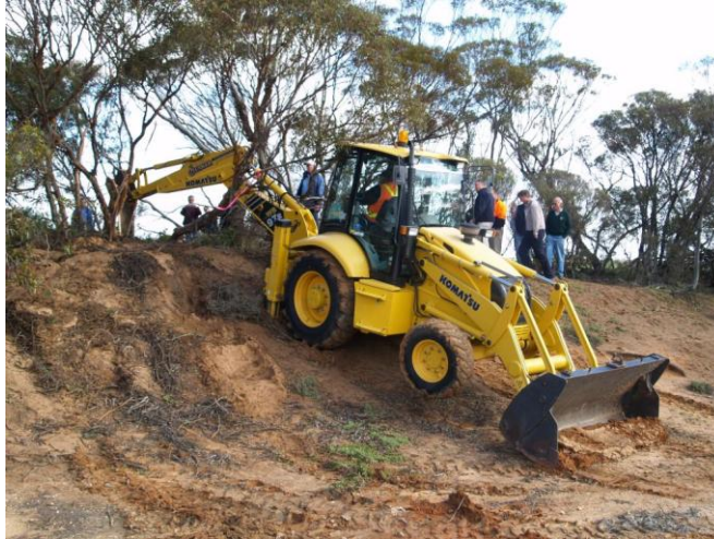
Figure 1. Demonstration of back-hoe at Smithville road field day. Steep sand-ridges and low vegetation make access to warrens difficult. A smaller Bobcat back-hoe was used in the main demonstration trial.
