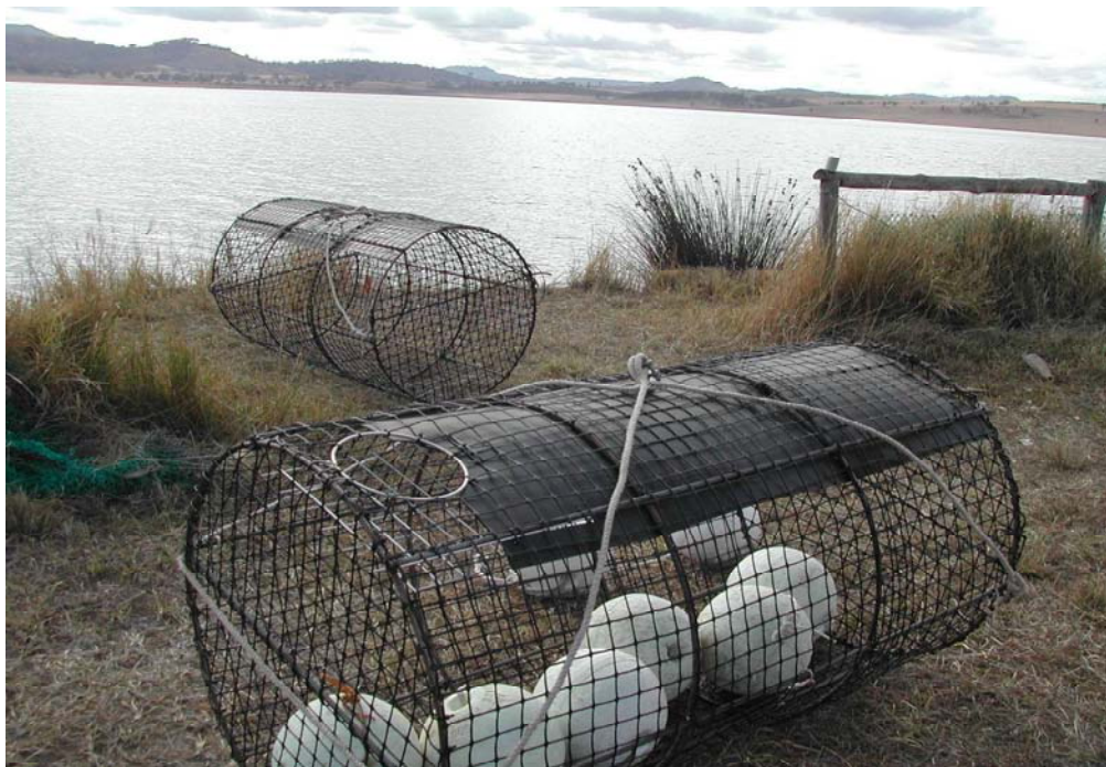
Figure 2. Envirotrap showing escape aperture for air-breathing animals.
