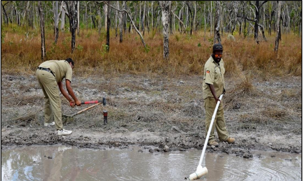
Rangers use the metal tubes, caps and hammers to collect soil samples (left) and an extended handle to collect water samples (right).
