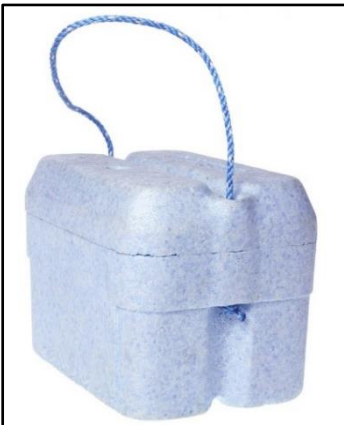
Figure 5: An appropriate Styrofoam container for couriers samples. Using dry ice will keep your samples frozen during transport and won't leave behind any residue (melted water), as it evaporates as carbon dioxide gas once it 'melts'.
