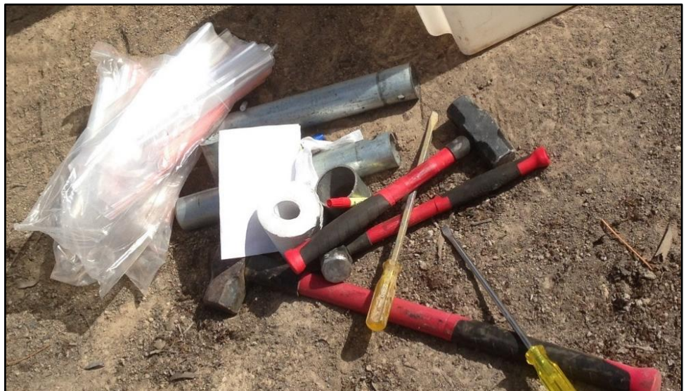
Some of the tools needed for soil sampling: snap lock bags, metal tubes, metal caps for the tubes, small and large hammers and screwdrivers.
