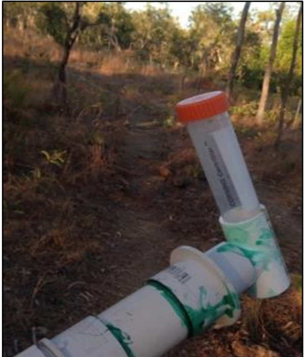
Figure 4: Ensuring all samples are correctly labelled with site, sample and date is critical. This 50 ml falcon tube is ideal for sampling water and recording site information.
