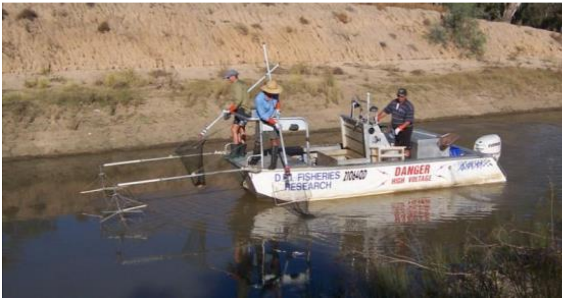
Figure 13: Large electrofishing boat with the Wisconsin array set-up for the anodes. Carp catches were increased in most water bodies by adding a single long wire to the centre of each array.
