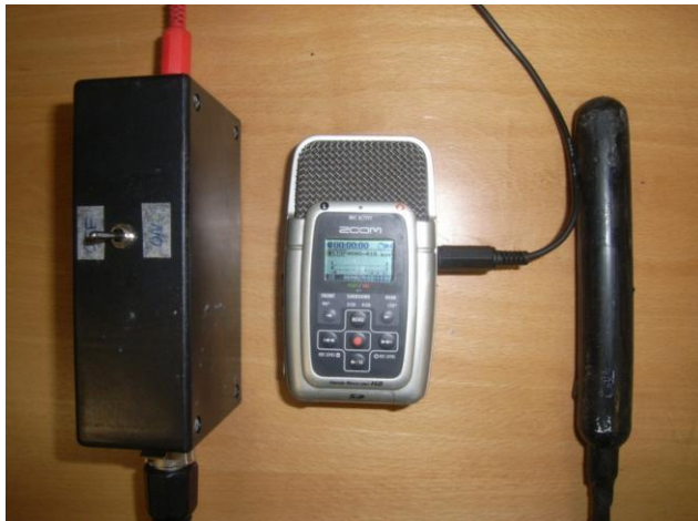
Figure 4. The underwater sound recording system. Zoom digital recorder (centre), 9V power supply for hydrophone (left) and AQ-18 hydrophone (right) (Photo: SARDI).
