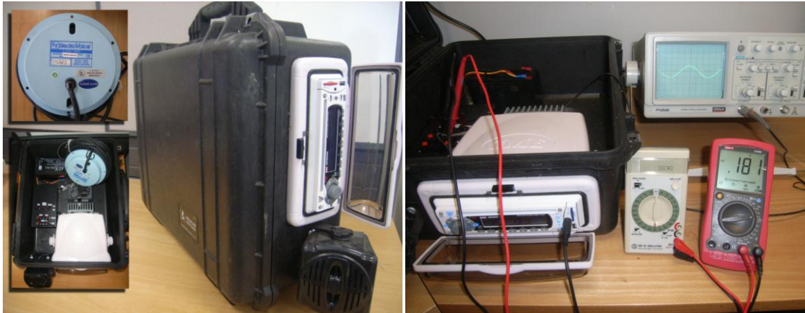
Figure 5. Acoustic sound playback system housed in a pelican case and the UW30 underwater speaker (left). Characterising the frequency response of the playback system (right) (Photo: SARDI).
