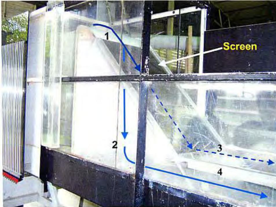
Figure 2: Two dimensional model trial of Coanda screen.
