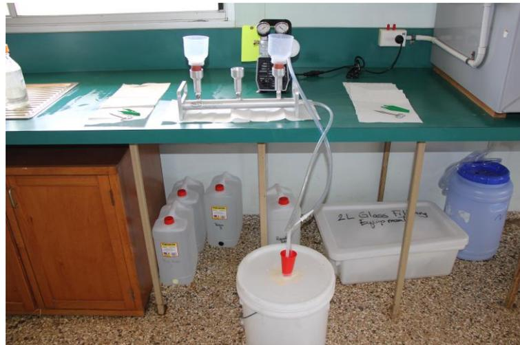
8. Set up workstation for filtering sample – At each station place a clean paper towel with:
