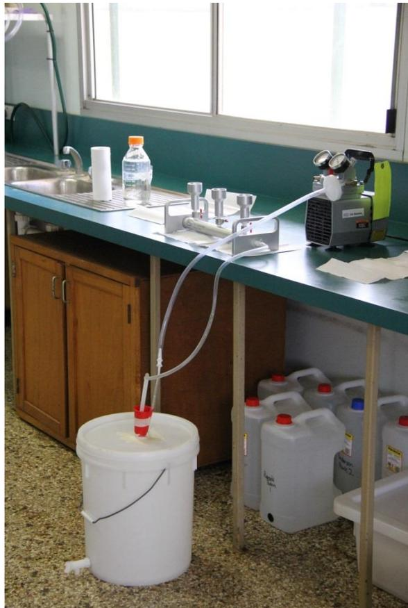
Photo: Laboratory set of filtration equipment ready for filtering eDNA water samples.
